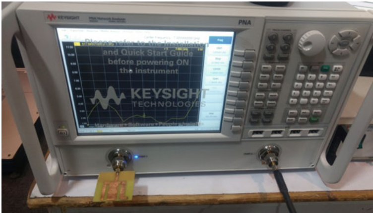
Fig. 14 Measurement setup of VSWR at 7 GHz
