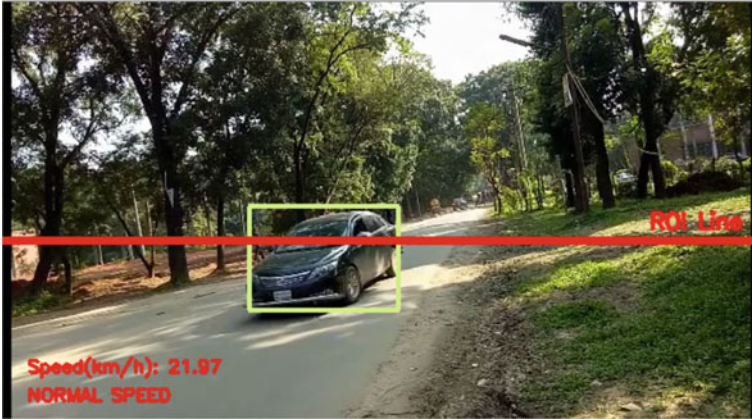
Fig. 2 Vehicle detection and speed estimation (normal speed)
