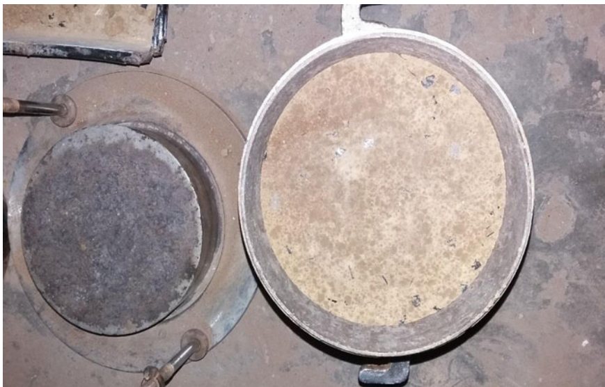
Fig. 2 CBR test mix composition in mould
