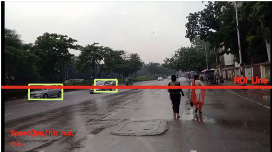
Fig. 4 The system could not estimate the vehicle speed due to multiple vehicle
