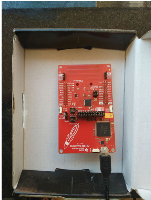
Fig. 44.4 Hardware setup of the receiver unit
