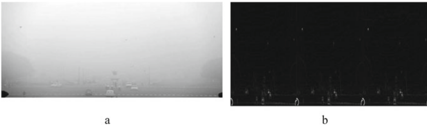
Fig. 10.5 a Original fog image, b sobel operator-based edge detection Image
