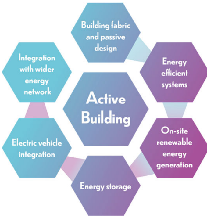
Fig. 5 Core principles of an active building [1]
