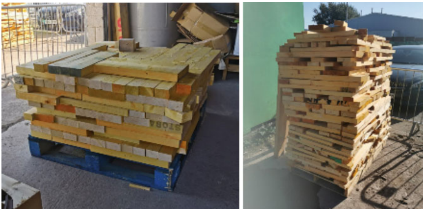
Fig. 12 Offcuts/waste timber neatly stacked ready to be burnt in the biomass boiler (authors image 2019)
