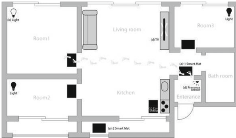
Fig 10 Smart mats installation scenarios. Laid at entrance (a)-1, each room and a place with flaw in security (a)-2.
