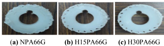
Fig. 12 Immense wear of driven gears at 1.6 Nm torque
