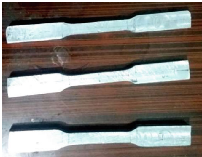
Fig. 2 Tensile bar specimen prepared by using milling machine
