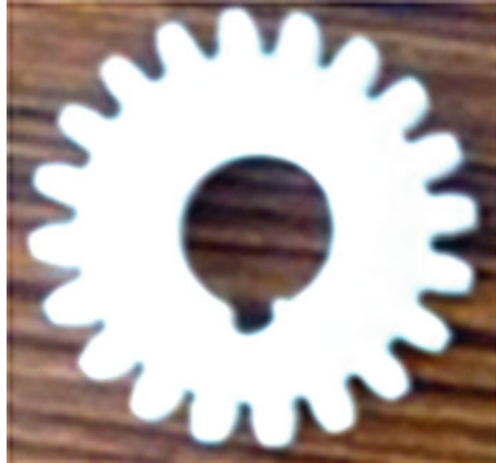
Fig. 1 Fabricated PA66 spur gear
