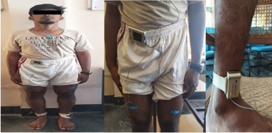
Fig. 1 Subject equipped with set of sensors, sub-recorders, and a main recorder
