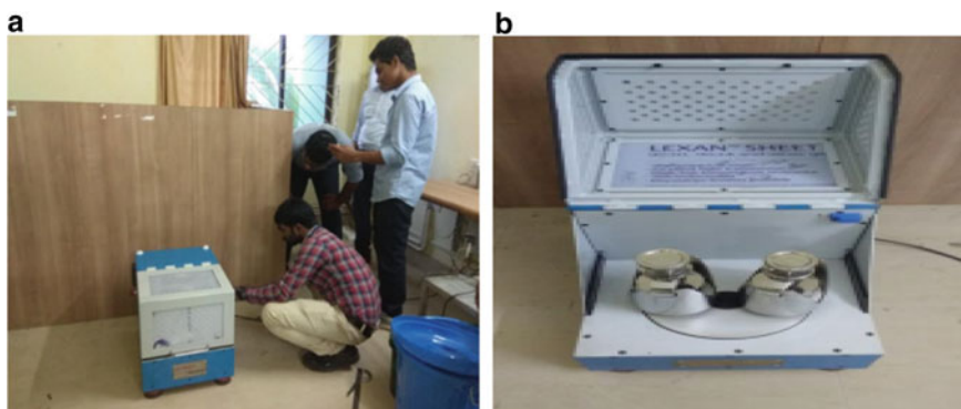
Fig. 12.2 a Ball mill grinder setup b ball mill grinder jar
