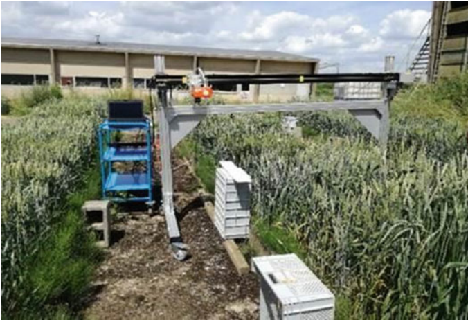
Fig. 14.2 Use of Hyperspectral NIR imaging for crop status monitoring ( Source CRA-W )
