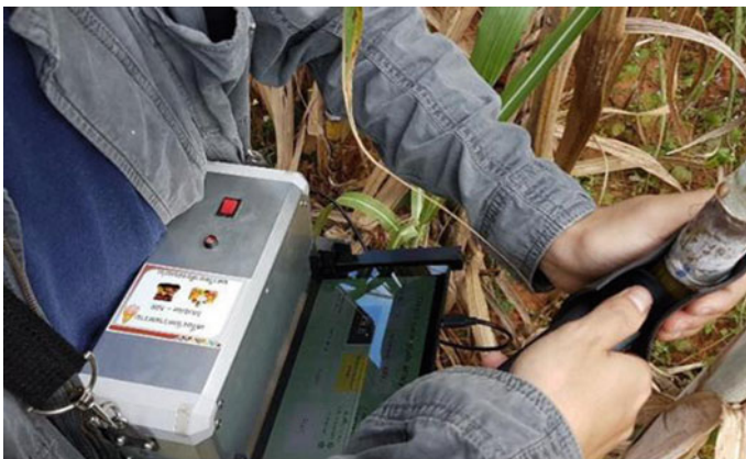
Fig. 17.4 Direct scanning of cane stalk using portable NIR instrument (P-TF1, HNK Engineering Co., Ltd., Iwade, Japan)
