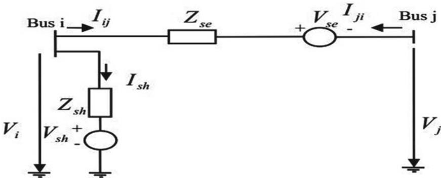
Fig. 1 UPFC configuration model
