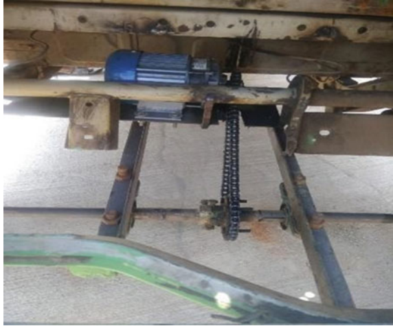
Fig. 3 BLDC motor coupled with sprocket wheel
