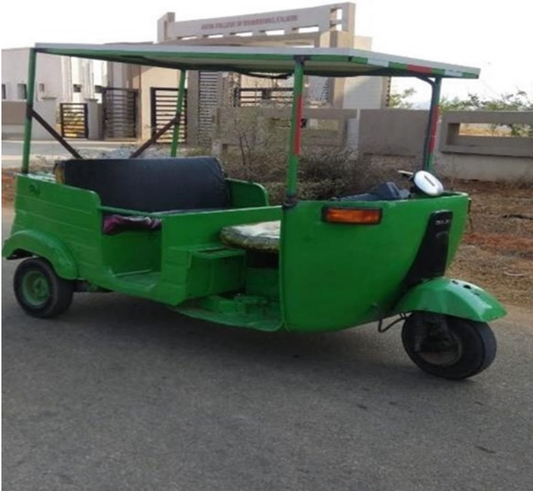
Fig. 5 Solar-powered electric vehicle that has been designed and implemented
