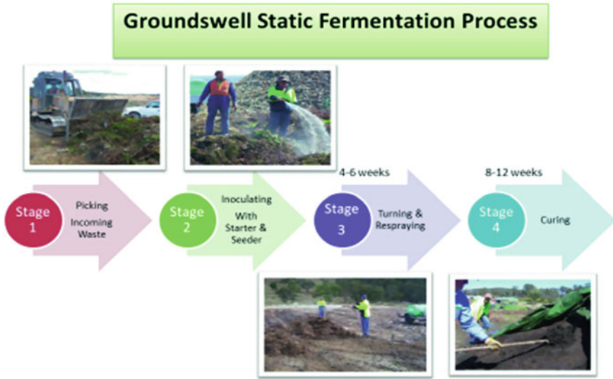
Fig. 4 Groundswell static fermentation process—Graphics courtesy of Ken Bellamy, Founder of VRM
