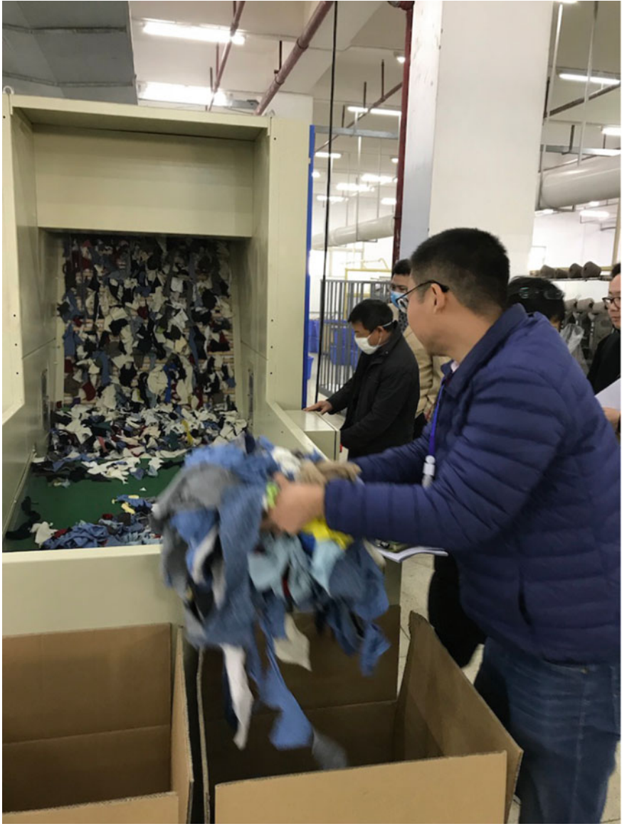
1. Cut up pieces of used apparel are fed into a shredding machine
