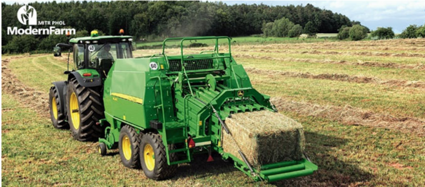
Fig. 7 Baler for cane leaves (Source http://www.mitrpholmodernfarm.com )
