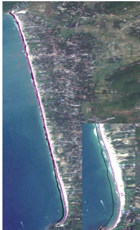
Fig. 8 The dotted line corresponds to the initial shoreline position, the dashed line illustrates the shoreline position for the case that Groyne 2 is considered impermeable, and the solid line shows the shoreline position for permeable groyne conditions at Groyne 2 impermeable, and the solid line shows the shoreline position for permeable groyne conditions at groynes 1 and 2
