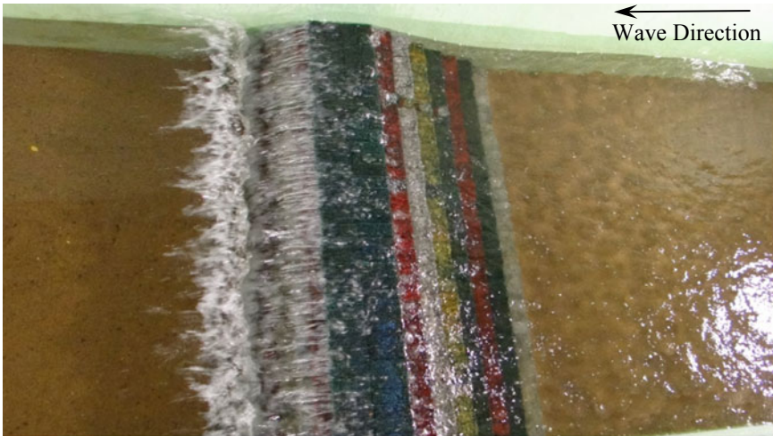
Fig. 4 Snapshot showing stability tests on emerged reef breakwaters
