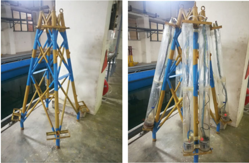
Fig. 3 Jacket model without buoyancy tanks (left side) and after attaching buoyancy tanks (right side)
