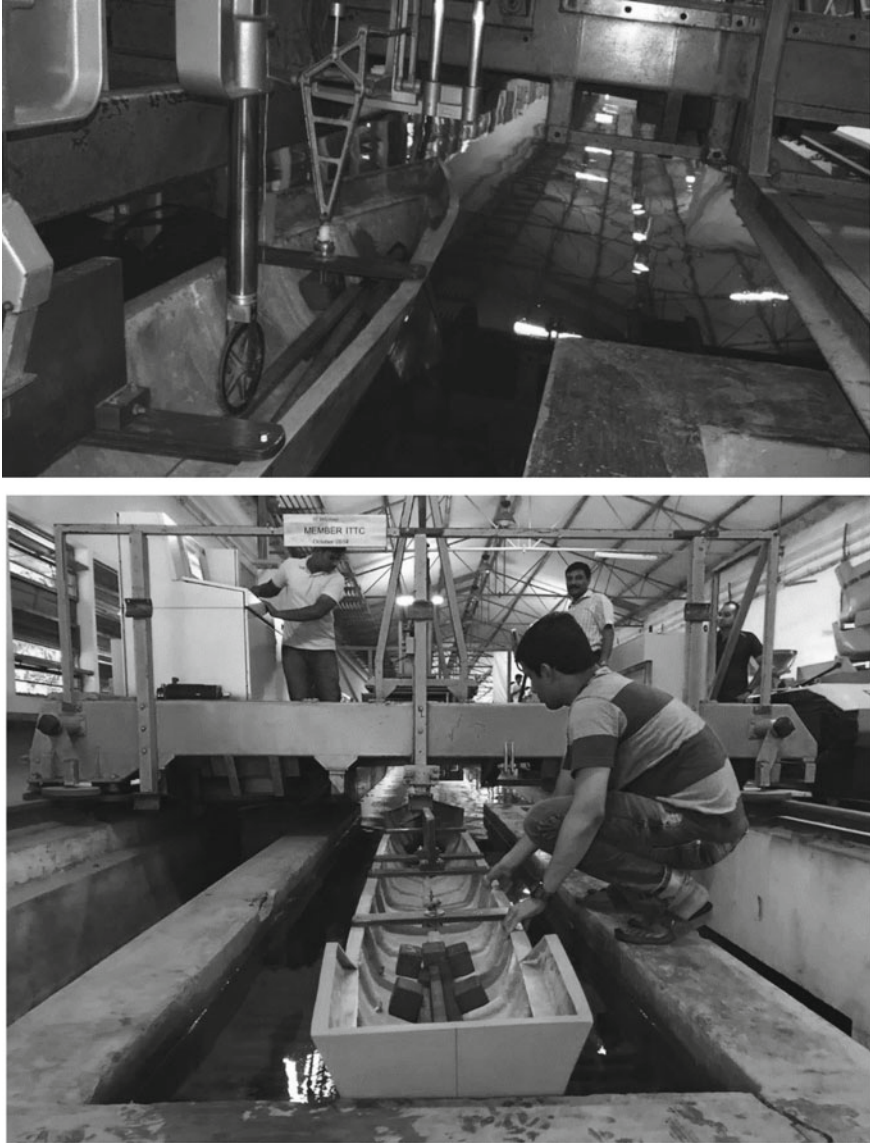
Fig. 3 Experimental setup in towing tank
