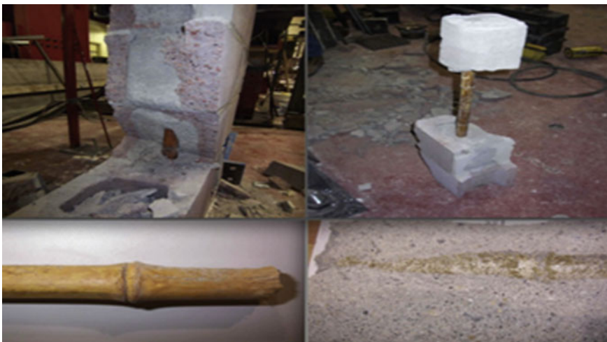
Fig. 9 Typical bamboo bond in-wall specimens [37]
