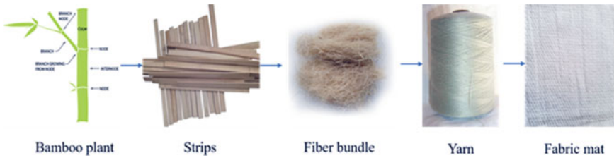
Fig. 1 Process of making bamboo fabric mats
