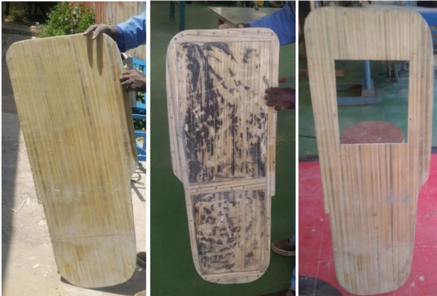
Fig. 6 Development of a car door prototype from a bamboo fiber composite [20]
