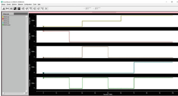
Fig. 14 Transient response of multiplexer
