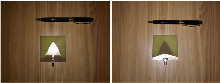
Fig. 8. Fabricated prototype of Antenna 3
