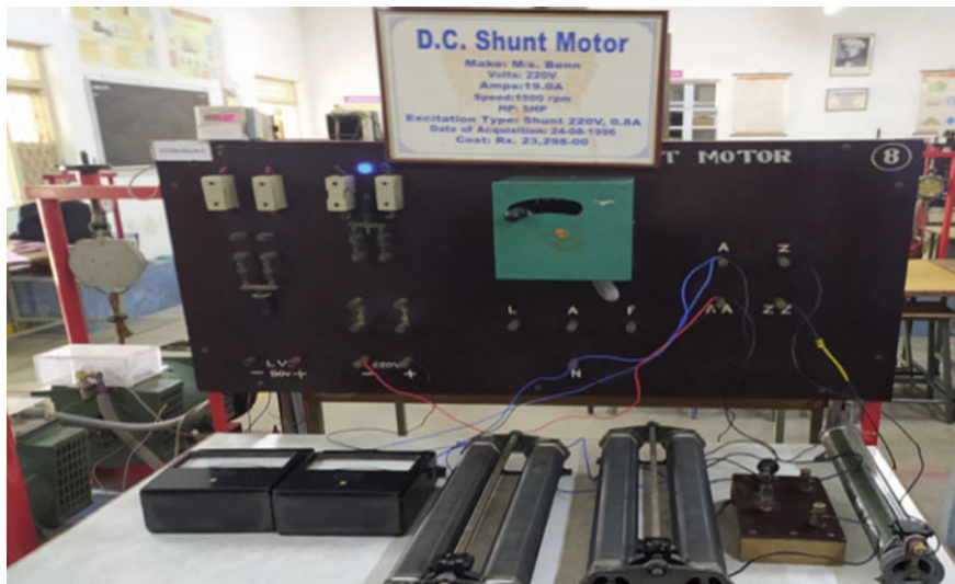
Fig. 3 Experimental setup of retardation test with field excited separately
