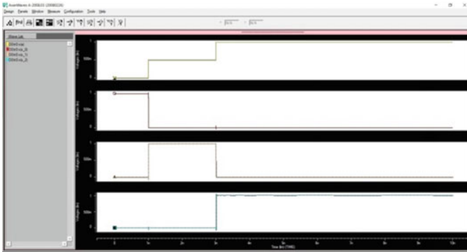
Fig. 11 Transient response of TDECODER
