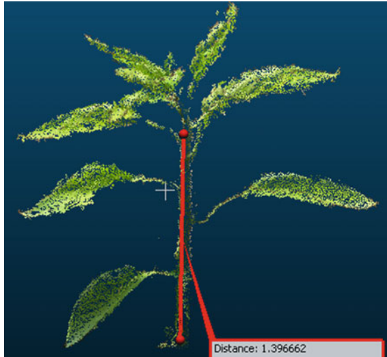
Fig. 3 The approximate calculation of stem height from the reconstructed 3D model
