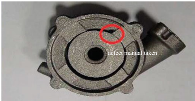
Fig. 3 MNF defect in diffuser area Problem
