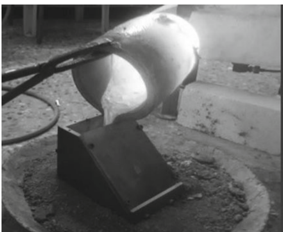
Fig. 3 Pouring mixture MMCs in wedge-shaped die
