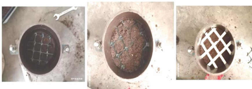
Fig. 1 CBR with geogrid and PVC grid
