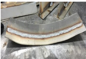
(a) Welding with distortion
