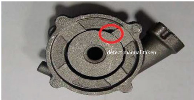
Fig. 3 MNF defect in diffuser area Problem
