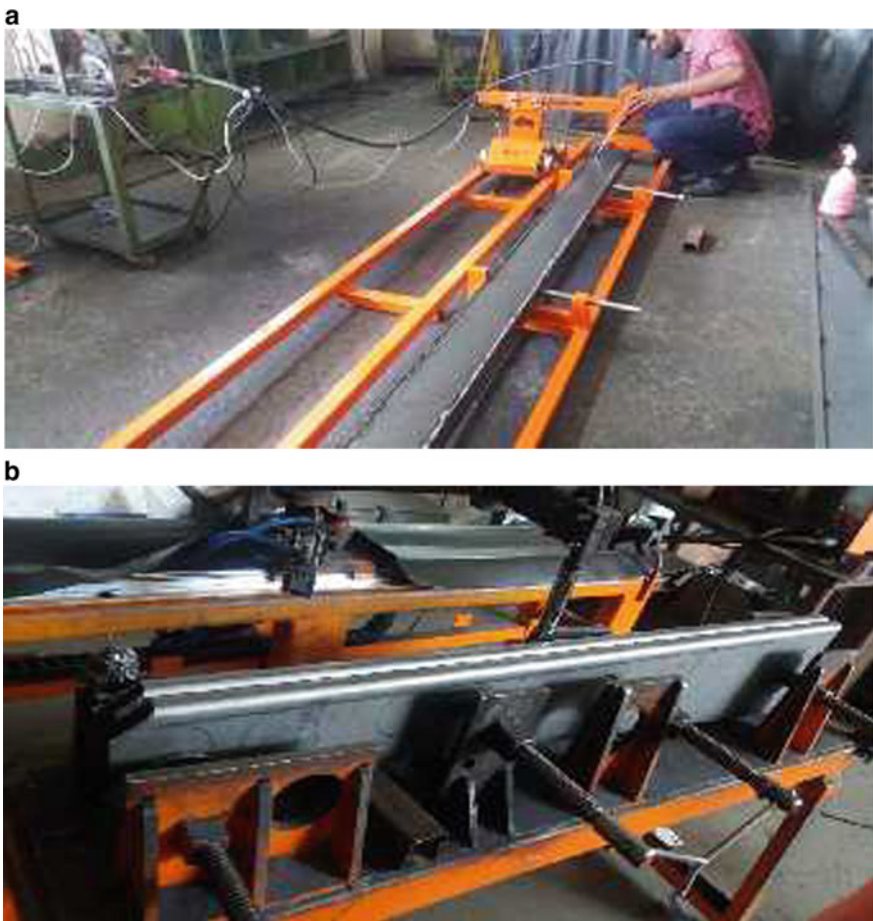
Fig. 1 a Welding fixtures without work piece. b Welding fixtures with work piece
