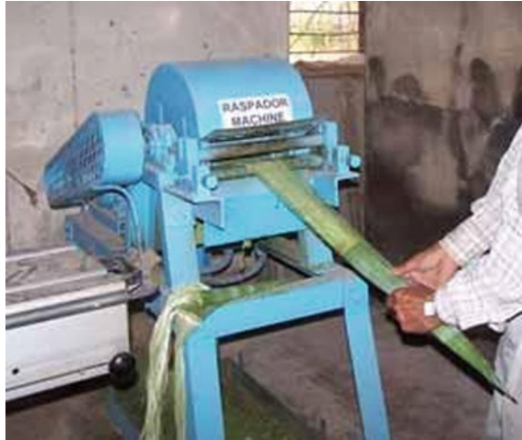
Fig. 1 Mechanical process of sisal fibre extraction using raspador machine
