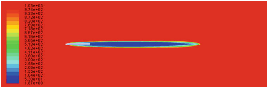
Fig. 15 Density contour for 12° with 1 mm cavitator disk 60 m/s velocity
