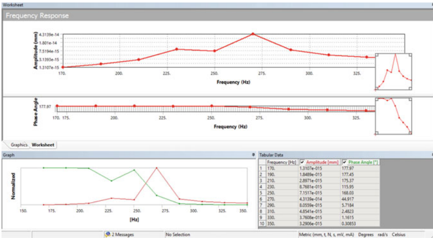
Fig. 6 Harmonic response analysis of the owl wing pattern turbine blade
