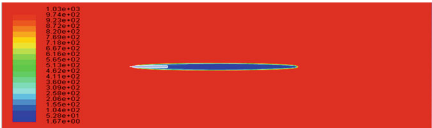
Fig. 18 Density contour for 15° cone cavitator at 55 m/s velocity
