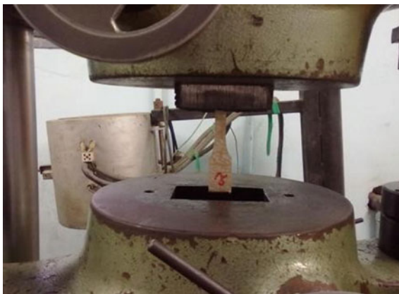
Fig. 10 Clamping of specimen in universal testing machine
