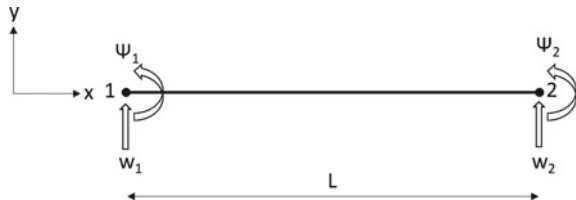
Fig. 8 Schematic of Timoshenko spectral beam element
