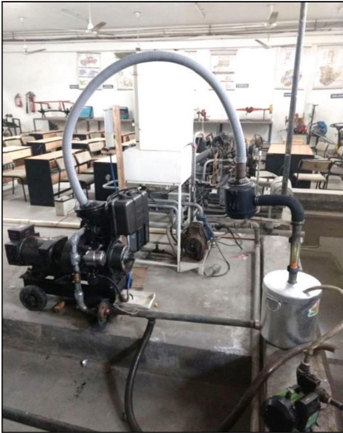
Fig. 2 Developed set-up with surge tank
