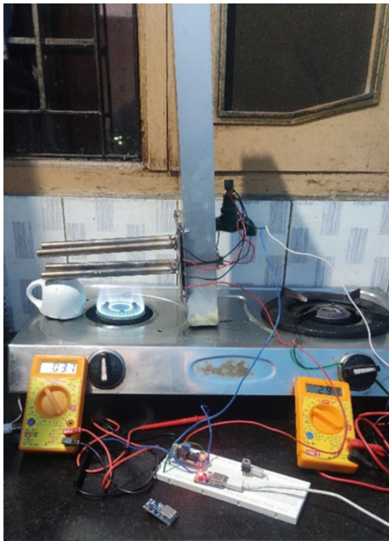
Fig. 7 Final model with booster circuit for WHRS system
