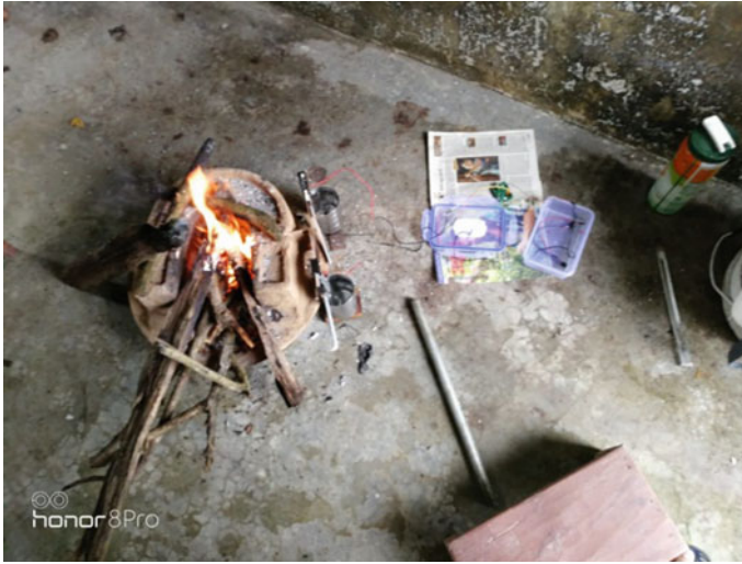
Fig. 3 Prototype model using copper plates on conventional chullah
