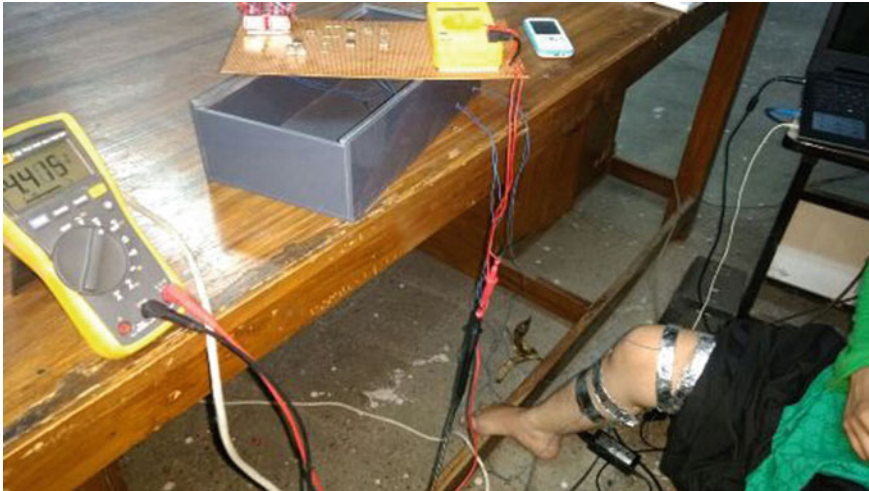
Fig. 11 Experimental setup for impedance analysis
