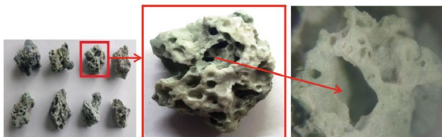
Fig. 2 EAF aggregate and its microscopic view showing pores [36]
