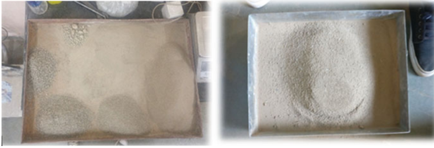
Fig. 3 Sieving of fine aggregate to adhere to zone II (left). Powder retained on pan (right)
