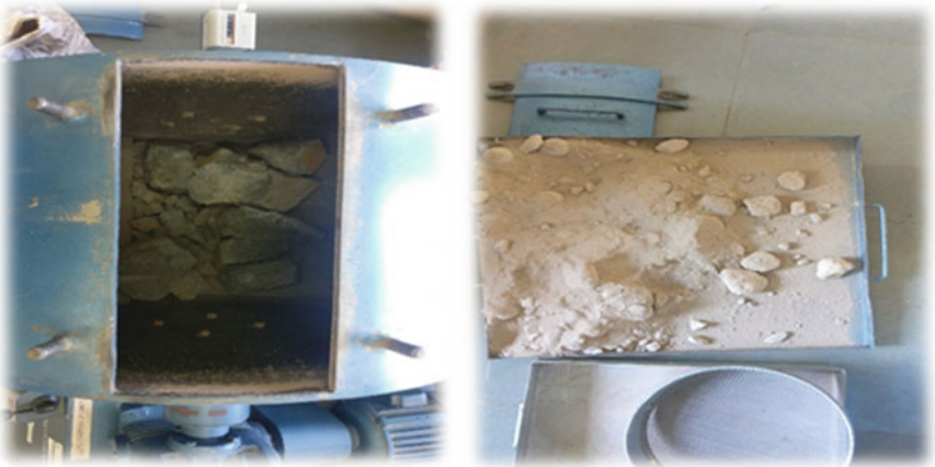
Fig. 2 Chunks of concrete in Los Angeles abrasion testing machine (left). Aggregate obtained after rotations (right)
