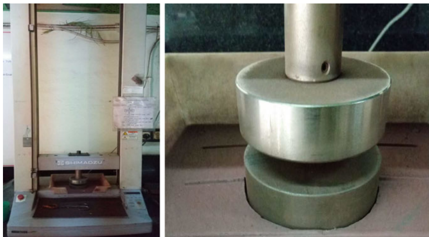
Fig. 3 CCS equipment and the pellet loading arrangement
