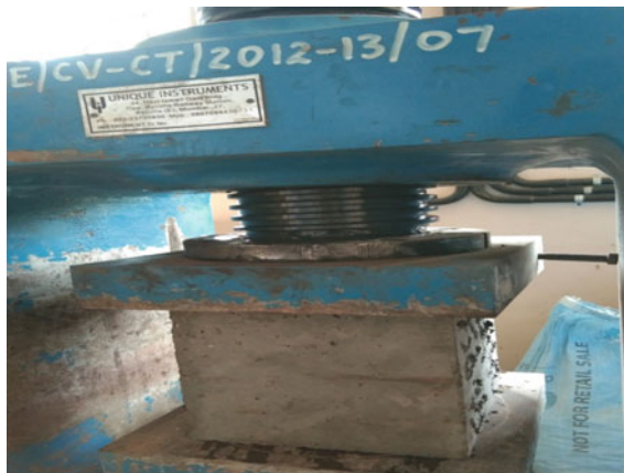
Fig. 1 Testing of concrete cube in CTM
