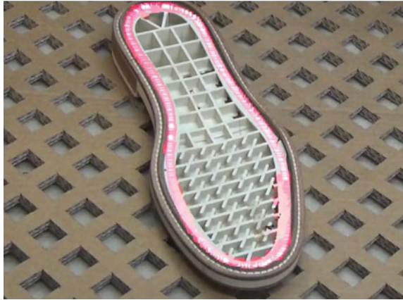
Fig. 12 Glue gun trajectory highlighted by means of a laser light connected to the glue gun nozzle
