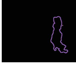
Fig. 11 Calculated contours from the binary image. The largest contour corresponds to a 6342.5 pixels and the smaller to only 0.5 pixels area
