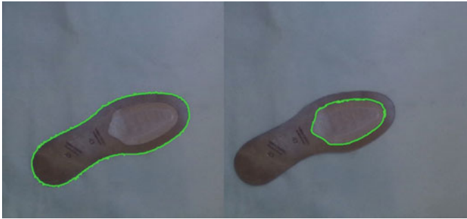
Fig. 15 Image elaboration: external and internal contour identification
