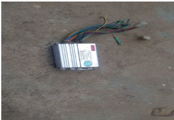
Fig. 5 Hub motor controller
