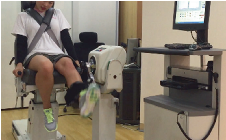
Fig. 1 Isokinetic strength test using dynamometer
