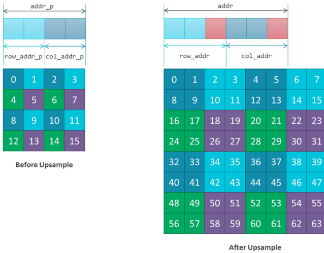
Fig. 10. An illustration of address mapping. Note that same color blocks in the result after upsample is represented the same origin pixel before the operation. (Color figure online)
