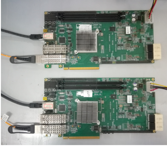
Fig. 2. Link error test system based on FPGA
