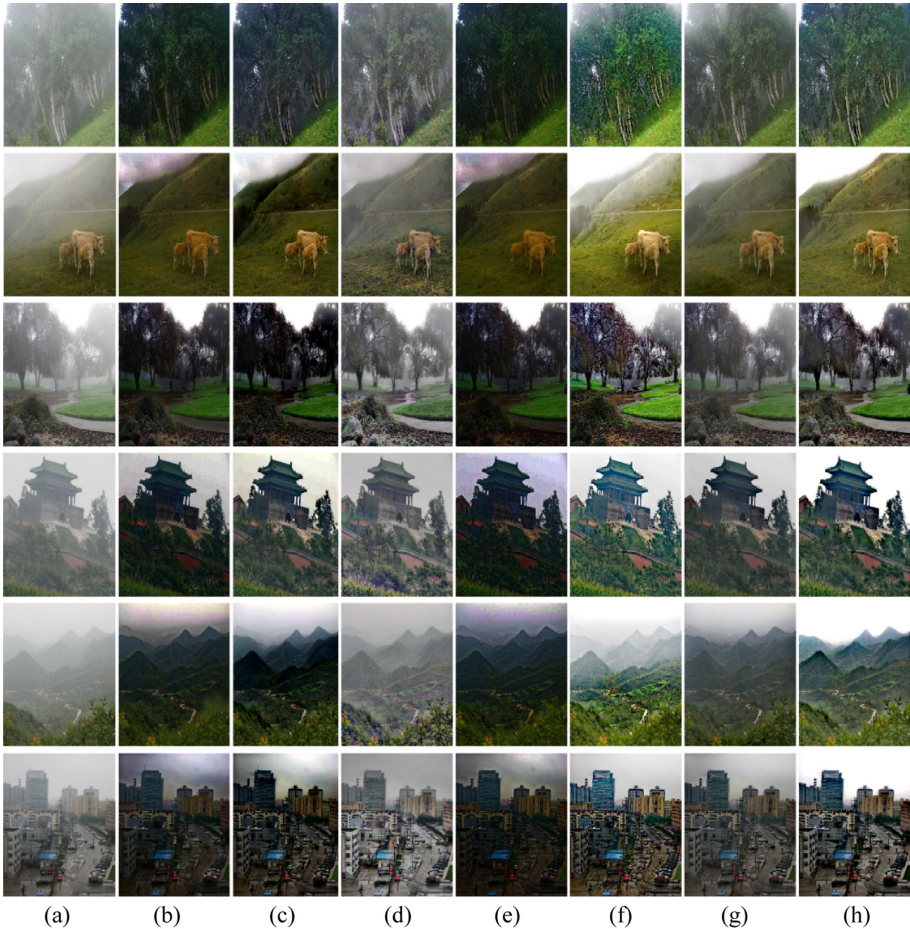
Fig. 4. Qualitative comparison of natural environment images. (a) The hazy images. (b) Ref. [7]. (c) Ref. [10]. (d) Ref. [1]. (e) Ref. [9]. (f) Ref. [30]. (g) Ref. [31]. (h) Our results.
