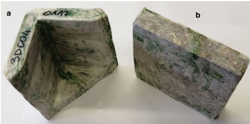
Fig. 3 Two different prototypes: angular element (a) and panel (b). The material had performed properly, according to the shape of the mold
