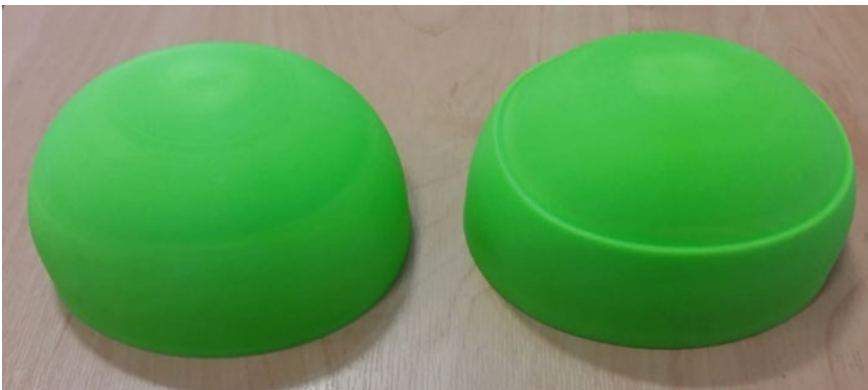
Fig. 7 Successfully printed scaled models: 2 mm overall thickness (left) and 4 mm edge thickened (right)
