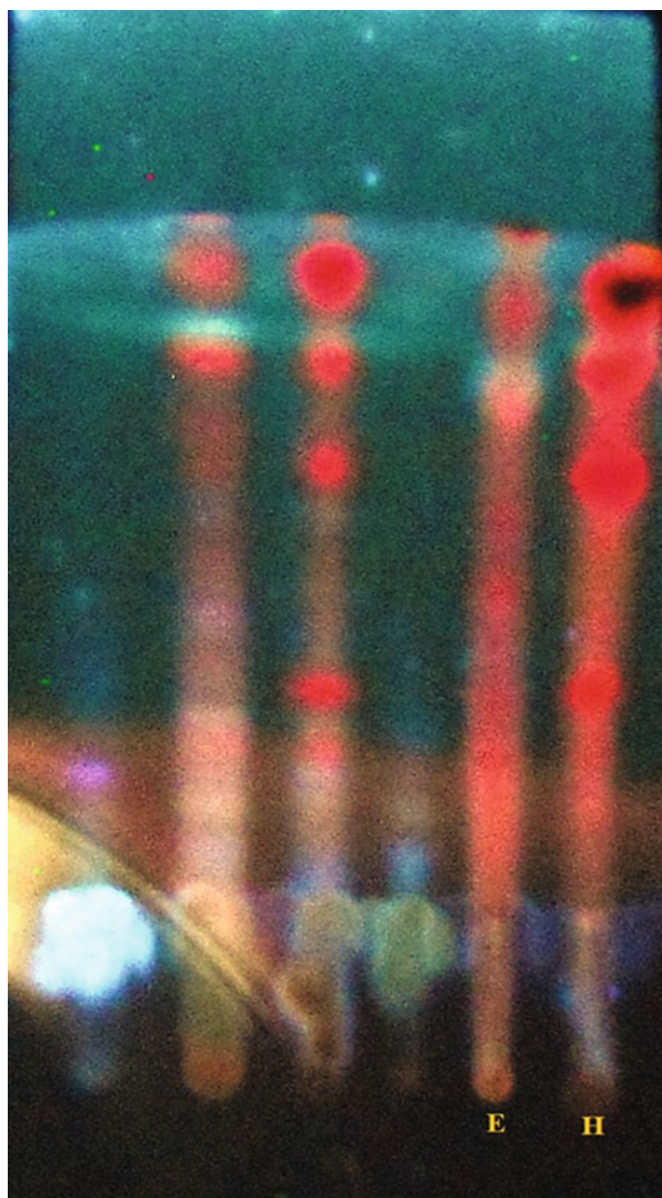
Fig. 47.2 TLC of O. debilis leaf extracts under 254 nm (E is ethyl acetate extract; H is hydro-alcoholic extract)
