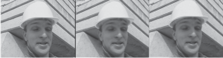
Fig. 8. Transmission quality in 80KBPS bandwidth (PSNR = 28.6 dB) (the left for the original image, and the middle for this paper decoding image, the right for Stamford scheme decoding image)
