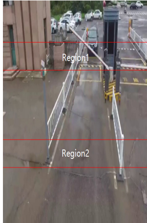
Fig. 3. Virtual loop detector design
