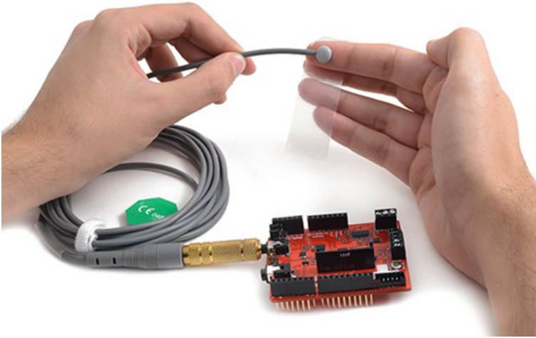
Fig. 22 Thermometer connection with processing unit
