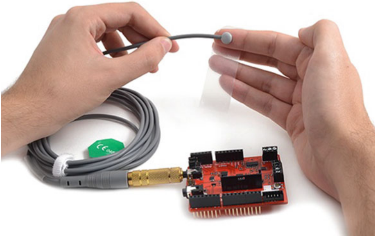
Fig. 22 Thermometer connection with processing unit
