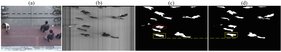
Fig. 2. a) LOIs, and temporal slice images from b) gray level, c) the initial line and d) the additional line. The red ellipse shows a special case of covering ellipse scheme in Sect. 2.2. The yellow rectangles show an example of direction determination in Sect. 2.4. (Color figure online)
