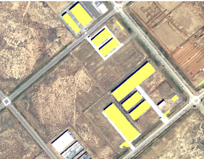
Fig. 7. Extraction results of blue roof buildings in the study area (Color figure online)
