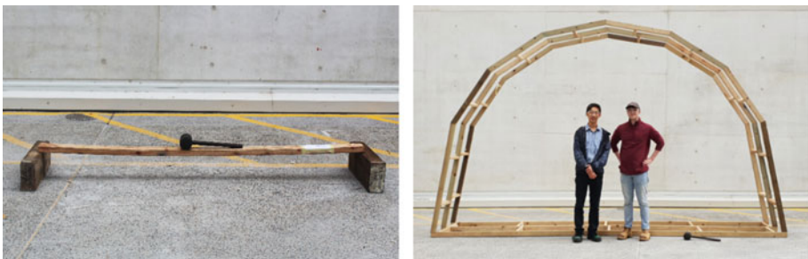
Fig. 1 Tested specimens: simply-supported beam (left) and semi-rigid timber frame (right)
