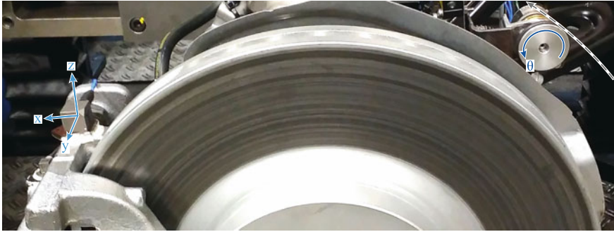
Fig. 4 Triaxial accelerometer mounted on caliper anchor and miniature rotation encoder with rubber ring pulley running on rim well
