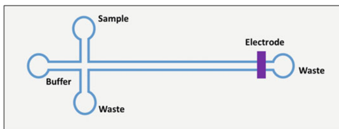
Fig. 7 Schematic representation of microchip design for biosensor applications in which samples are pre-treated, mixed with reagents and detection can be performed in one go either sequentially or simultaneously (Concept from: Arrigan 2015)
