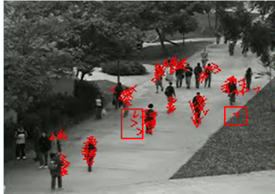
Fig. 1. Abnormal optical flow obtained by L-K pyramid optical flow method
