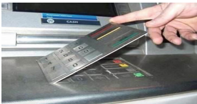
Fig. 2 Shows Keyboard overlays on ATM [24]
