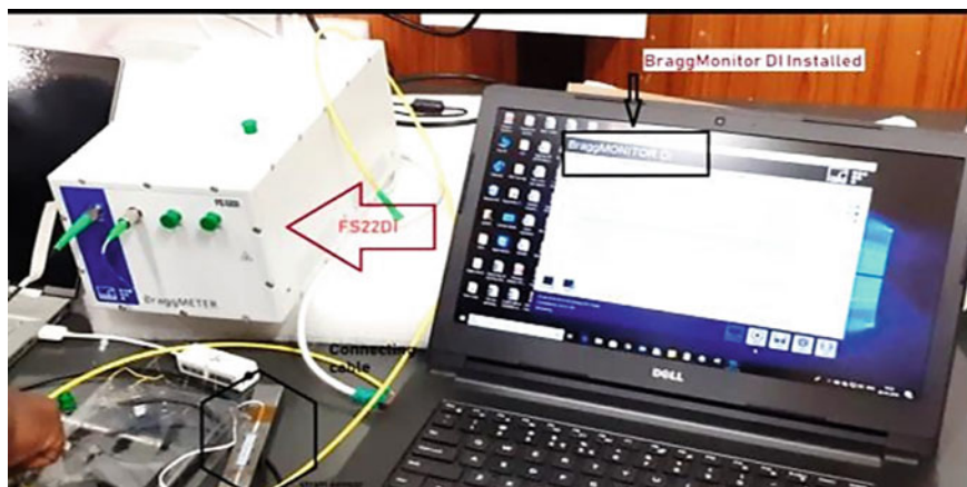
Fig. 3 Complete setup of FS22DI Bragg Meter DI with Installed software
