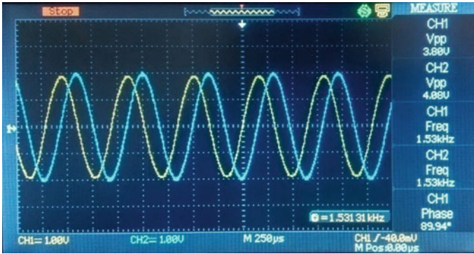
Fig. 3.9 Experimentally observed waveforms of V_1 and V_2 , f = 1.53 kHz
