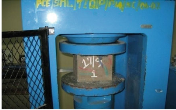
Fig.1 Cube under compression test
