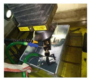
to decrease the gap between work and electrode. Thus, the process becomes more stable, and good MRR value is obtained with relatively good surface finish (Fig. 2).
