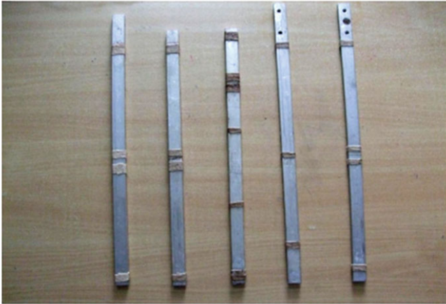
Fig. 1 Photograph of different aluminum crack beam specimens
