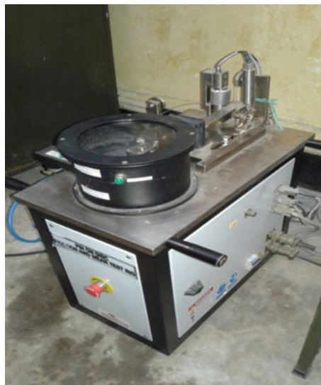
Fig. 1 Pin-on-disk friction and wear test rig
