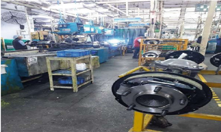
Fig. 1 Unchecked welding arc light passing through striped curtain
