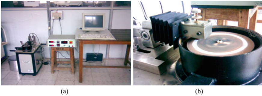
Fig. 3 Pin-on-disk setup for test
