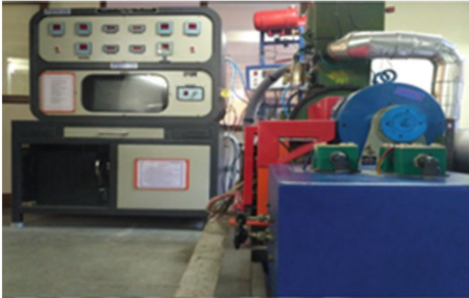
Fig. 1 Engine test rig with water cooling and computer-based data acquisition system
