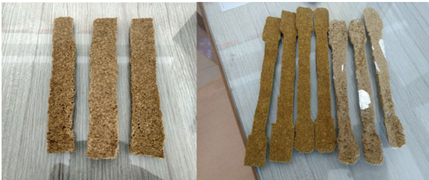
Fig. 1 Bio-composite developed as per ASTM D638
