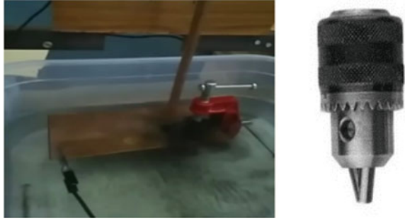
Fig. 6. Workpiece holder (left) and tool holder (right)
