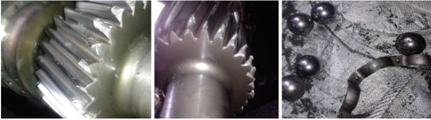
Fig. 6 Damaged intermediate gear and roller bearing
