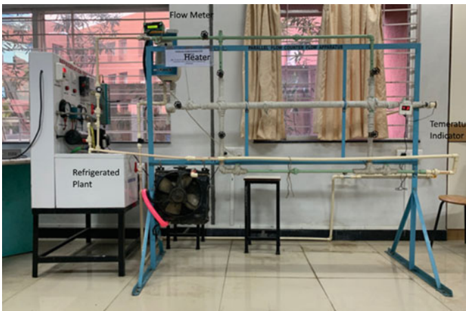
Fig. 1 Double pipe heat exchanger experimental setup
