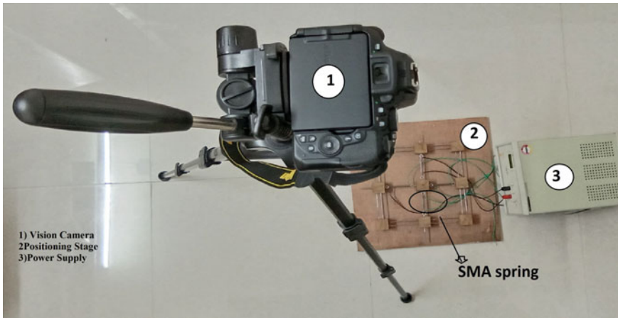
Fig. 3 Experimental setup of 4PP motion stager
