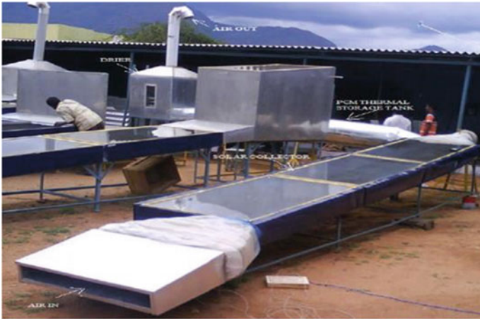
Fig. 4 Photograph of the indirect solar air dryer with Sunit [14]
