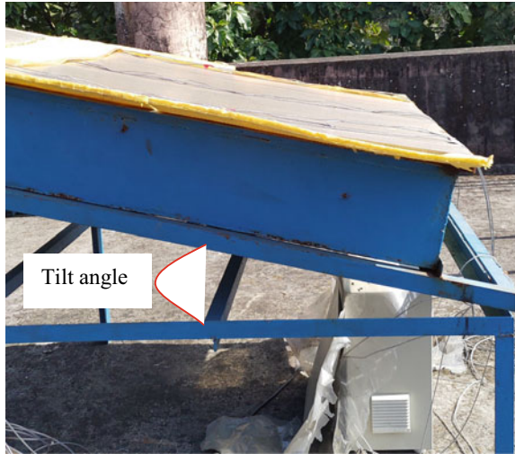
Fig. 3 Arrangement for sheet inclination (side view)
