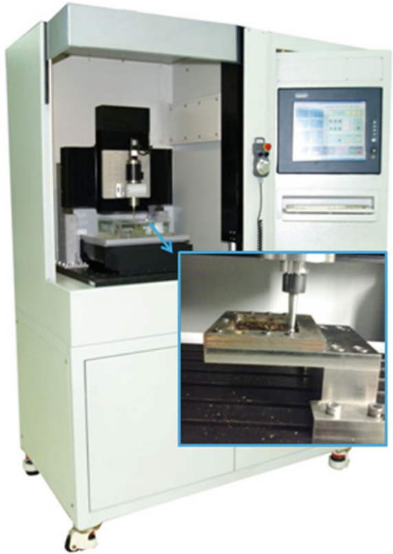
Fig. 1 Mickrotool DT-110 and typical fixture of SPIF
