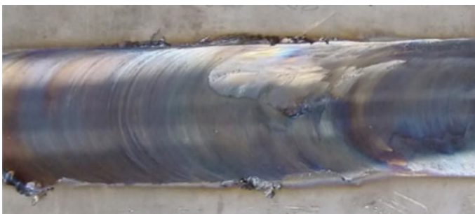
Fig. 2 FSW welded Inconel 718
