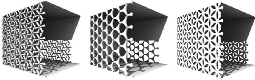
Fig. 6 Some examples of screen configurations simply using the symmetry of the wallpaper group (Constructed by Seoung Beom Park)
