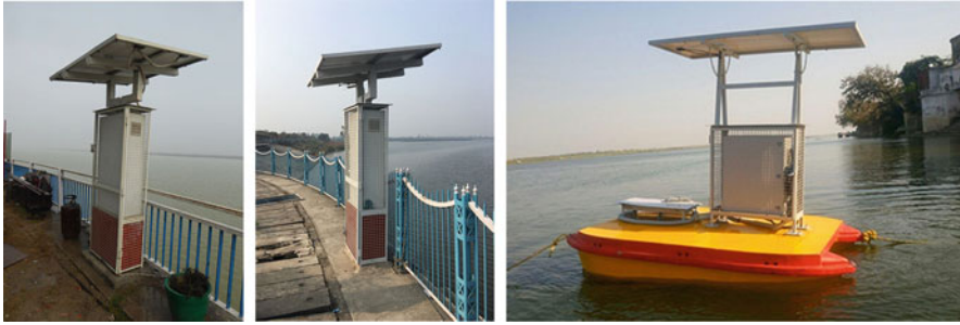
Fig. 20.4 Real-time water quality monitoring stations of CPCB
