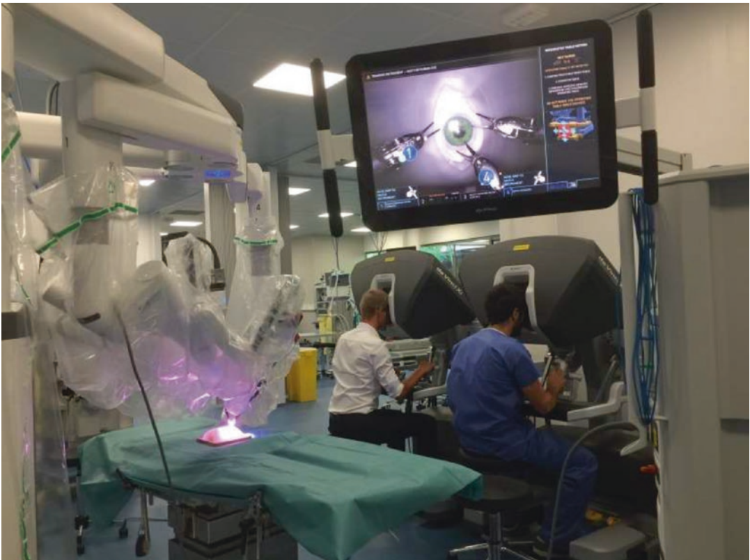
Fig. 40.3 da Vinci Xi surgical system being used in simulated strabismus surgery (photo from Bourcier T, Chammas J, Gaucher D, et al. Robot-assisted simulated strabismus surgery. Transl Vis Sci Technol. 2019;8(3):26)
