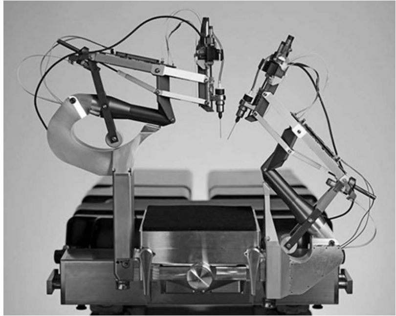
Fig. 40.4 PRECEYES Surgical System: a telerobotic surgical system developed by PRECEYES BV in the Netherlands. This is the only commercially available ophthalmic robotic surgical system (photo from de Smet MD, Stassen JM, Meenink TC, Janssens T, Vanheukelom V, Naus GJ, et al. Release of experimental retinal vein occlusions by direct intraluminal injection of ocriplasmin. Br J Ophthalmol. 2016;100:1742–6)
