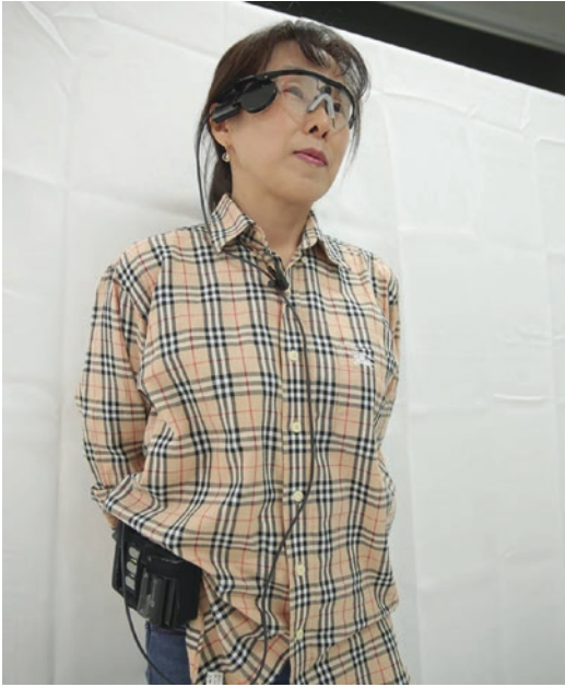
Fig. 34.2 Photograph of a patient wearing the Argus II retinal prosthesis system
