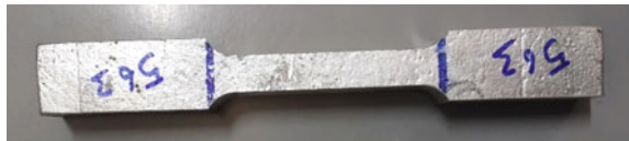
Fig. 3 Test sample before tensile test
