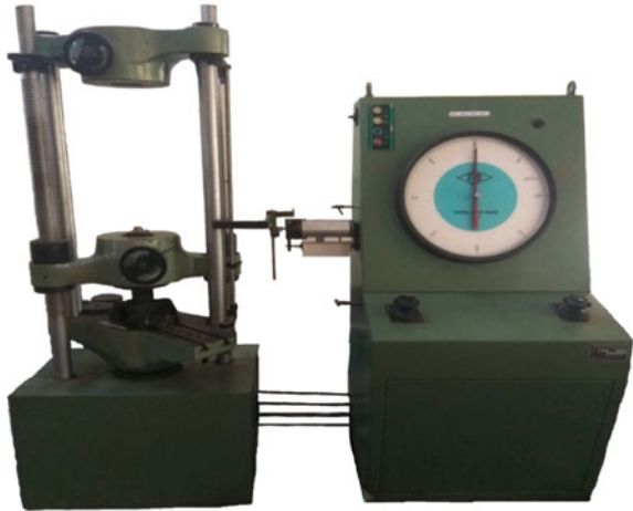
Fig. 5 UTM with special attachment of bending fixture of model: UTM 40 ton
