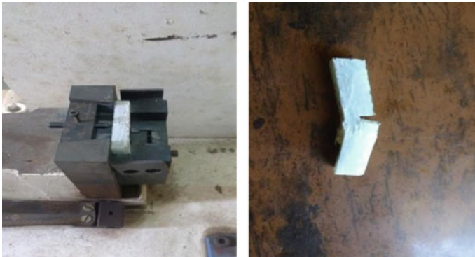
Fig. 7 Specimen before and after impact test
