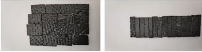
Fig. 5 MWCNT inclusion specimens for compression and impact test
