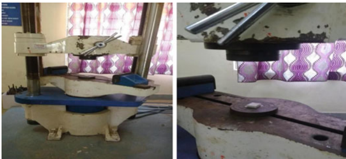
Fig. 5 Compression Testing for given GFRP sample
