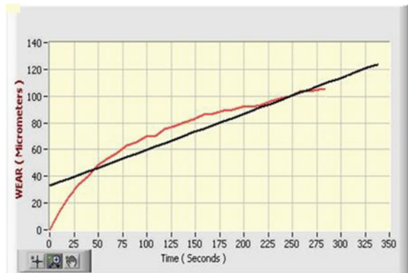
Fig. 7 Graphs for wear rate of powder metallurgy specimen at 2.5% of WC
