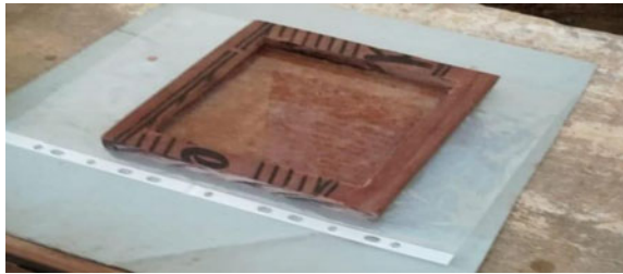
Fig. 2 Mould for fabricating a GFRP specimen
