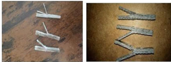
Fig. 9 Specimen subjected to Impact test with and without the inclusion of MWCNT
