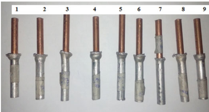
Fig. 4 Nine samples weldment of aluminium and copper
