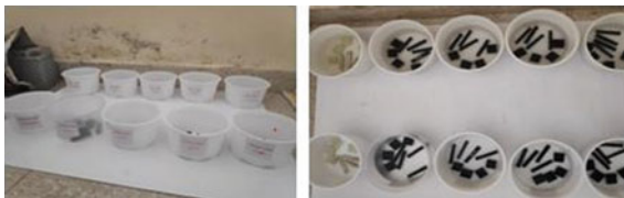
Fig. 10 Specimens Immersed in Normal water and Seawater for testing (impact and compression)
