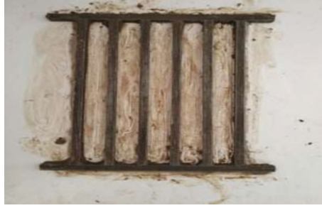
Fig. 2 Pattern for sample preparation (composite of (250 mm × 25 mm × 10 mm))
