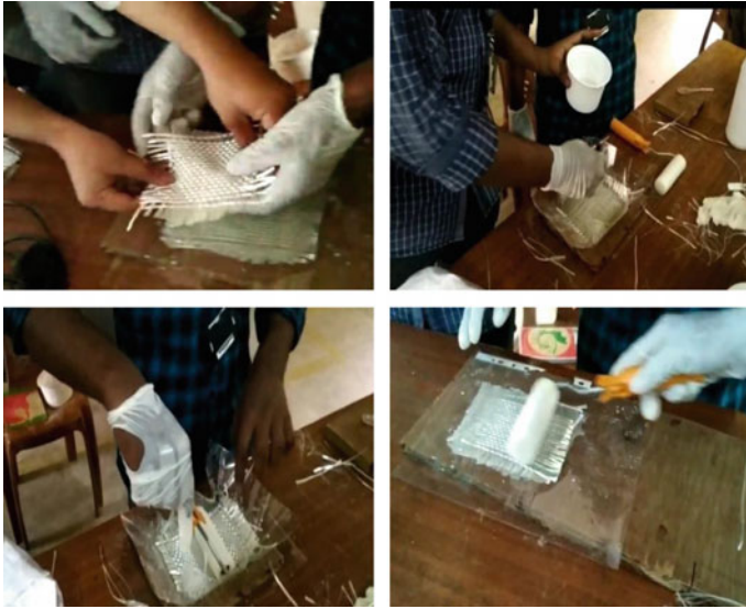
Fig. 4 Fabricating the specimen using hand lay-up technique
