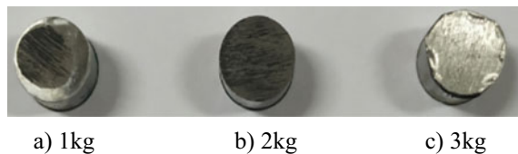
Fig. 3 304-Austenitic stainless steel pin specimens after wear test
