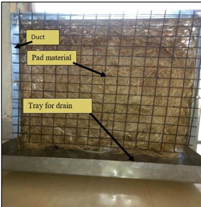
Fig. 3 Cooling pad material
