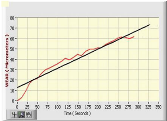
Fig. 9 Graphs for wear rate of powder metallurgy specimen at 7.5% of WC
