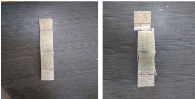
Fig. 8 Specimen before and after tensile test
