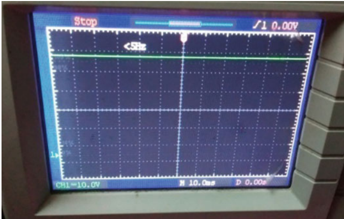
Fig. 11 Output voltage of SEPIC converter
