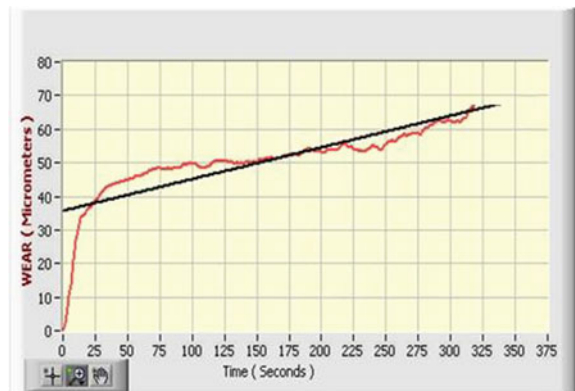
Fig. 8 Graphs for wear rate of powder metallurgy specimen at 5.0% of WC
